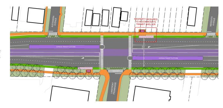
Figure 6-8 – Example Median BRT Bus Stop Layout - Lakefront Promenade
